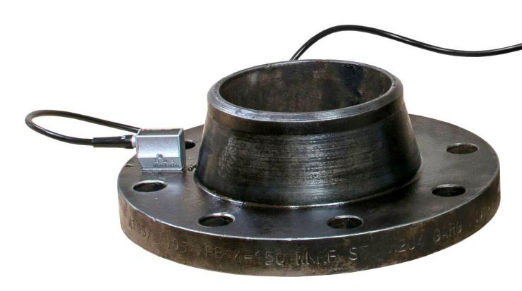
Detection and evaluation of the flange face corrosion with use of PA probe placed onto the flange
