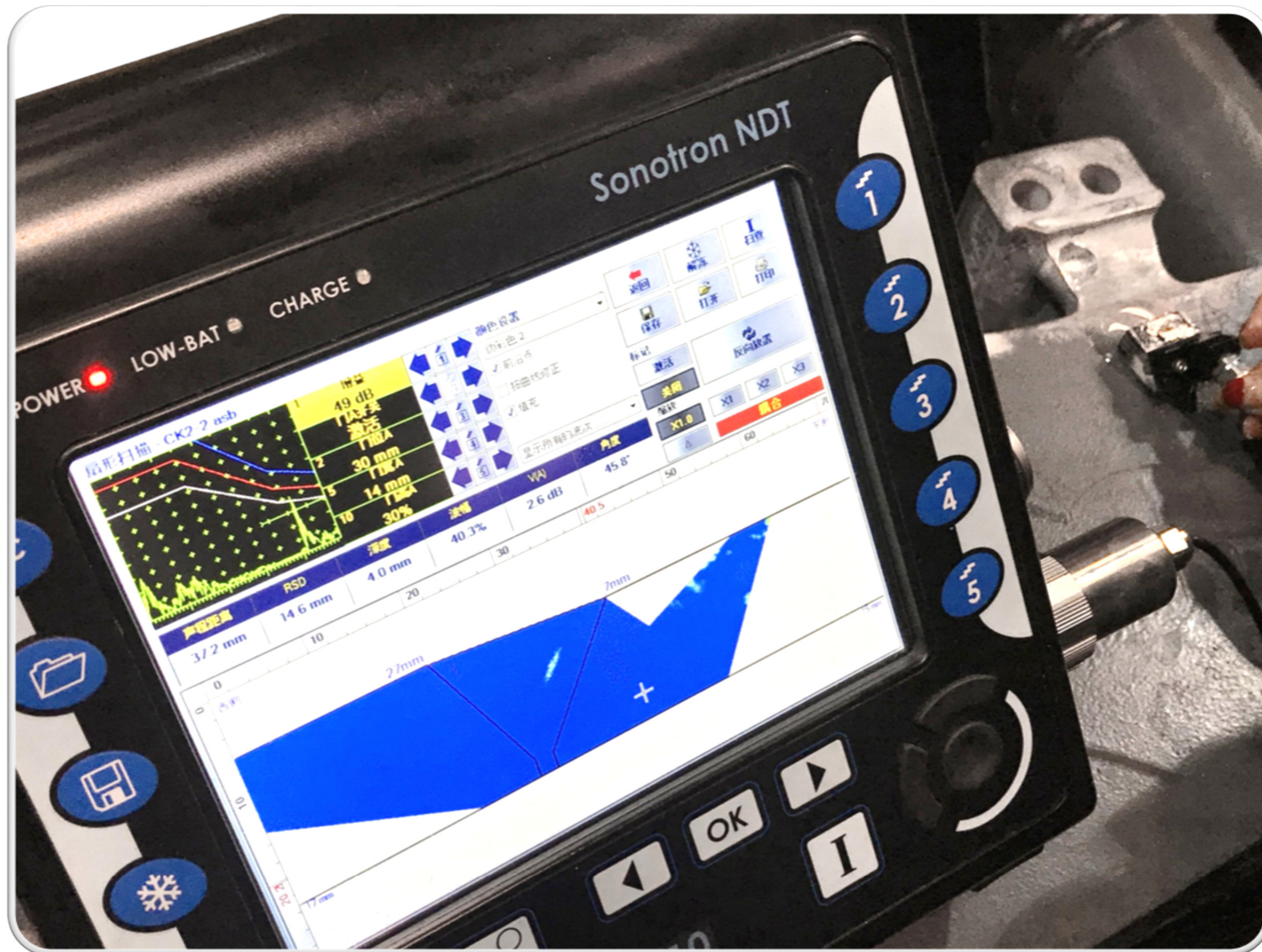
Inspection of the special weld in the train coupler
