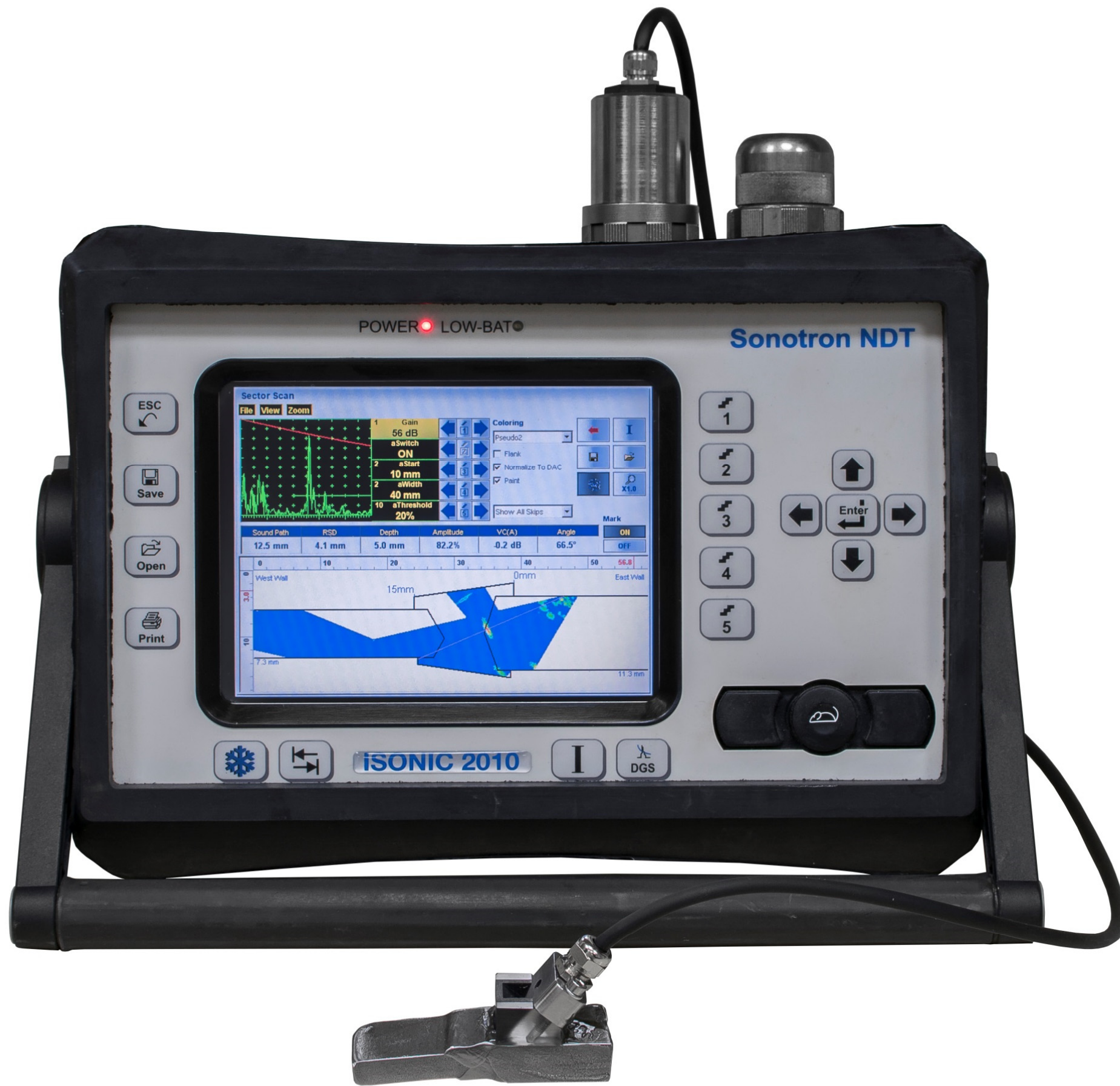
Inspection of the asymmetrical cross section butt weld between the rings with the different wall thickness – heavy machinery industry
