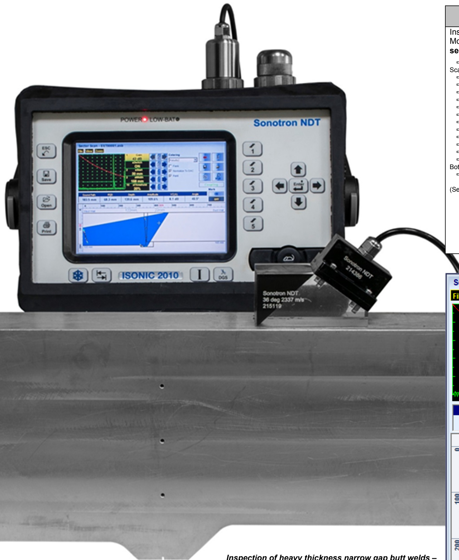
Inspection of heavy thickness narrow gap butt welds – calibration / performance demonstration block
