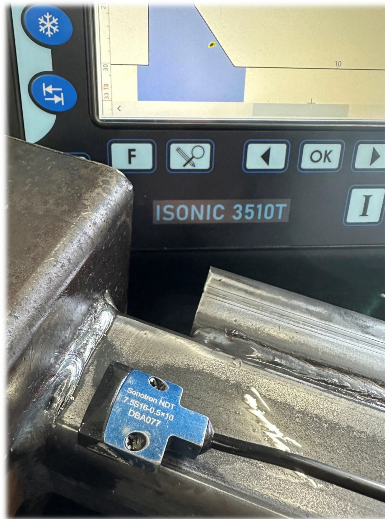
Structural straight corner weld between thin wall rectangle cross-section profiles
