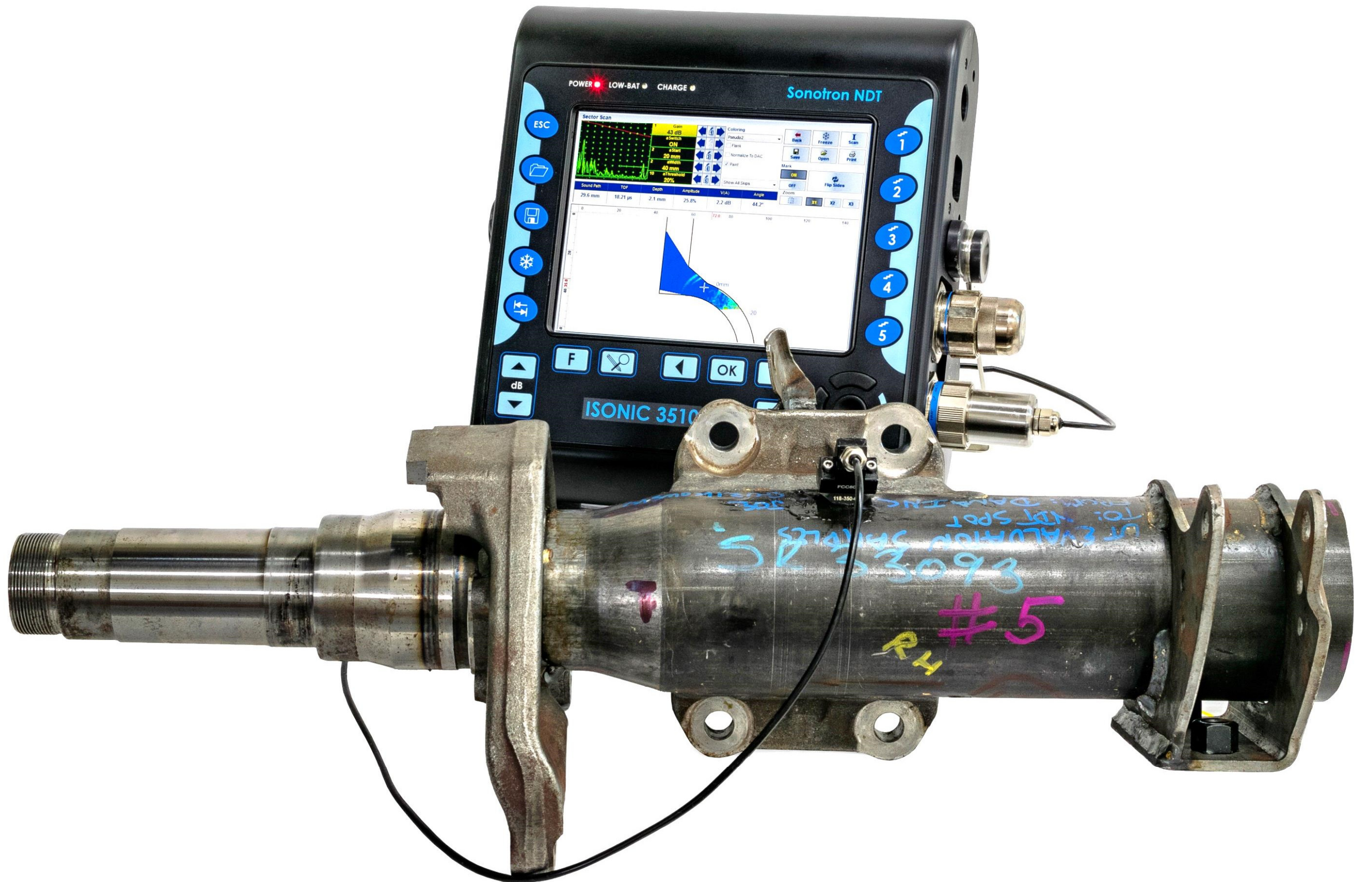
Shear wave inspection of the corner weld: automotive industry
