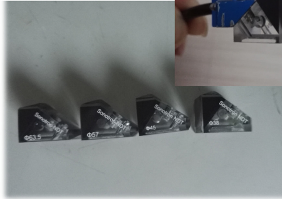
Inspection of nozzle weld through scanning above the nozzle tube
