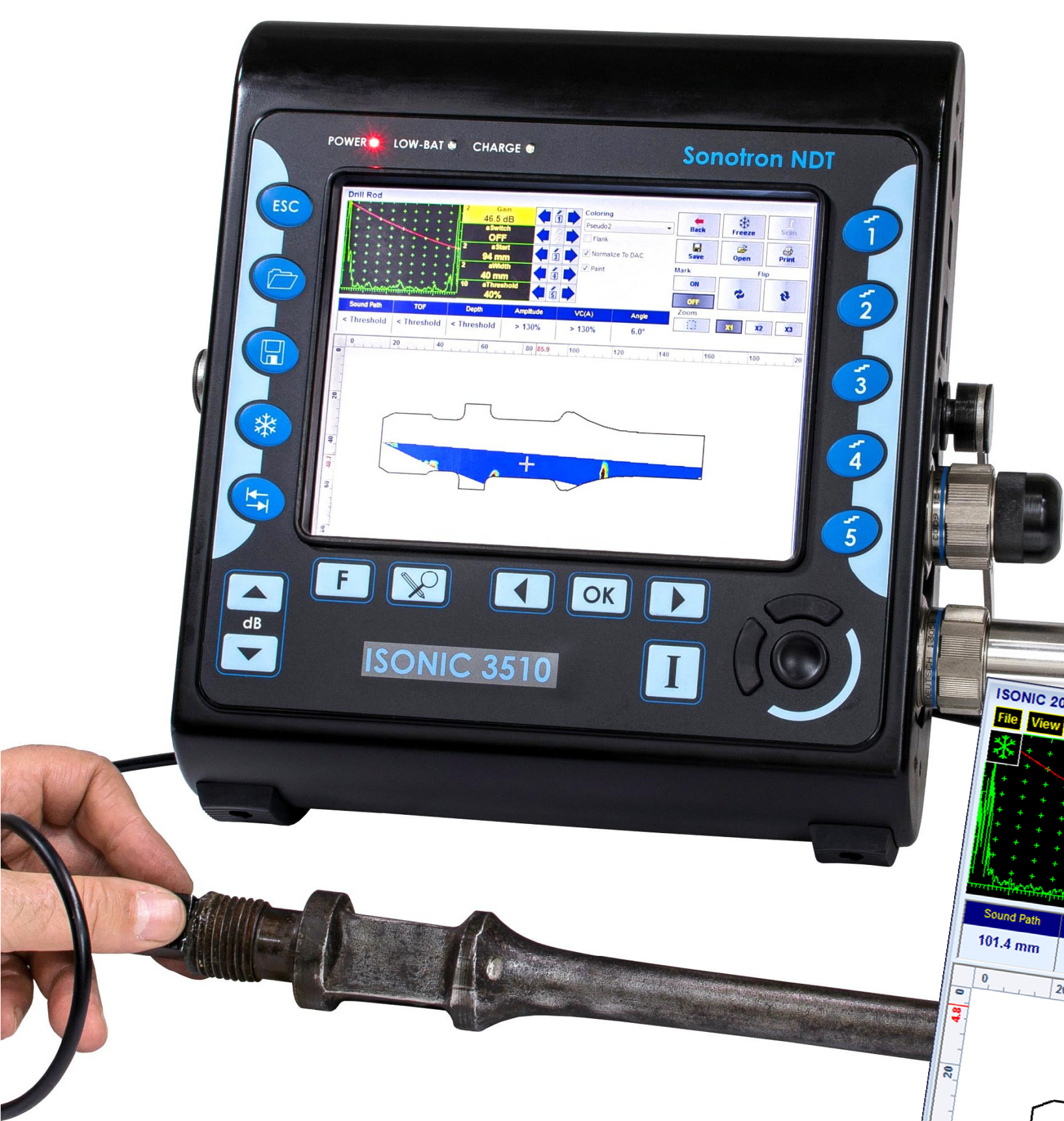
Inspection of the Drill Rod for the Transversal Cracks – Scanning from the End Side
