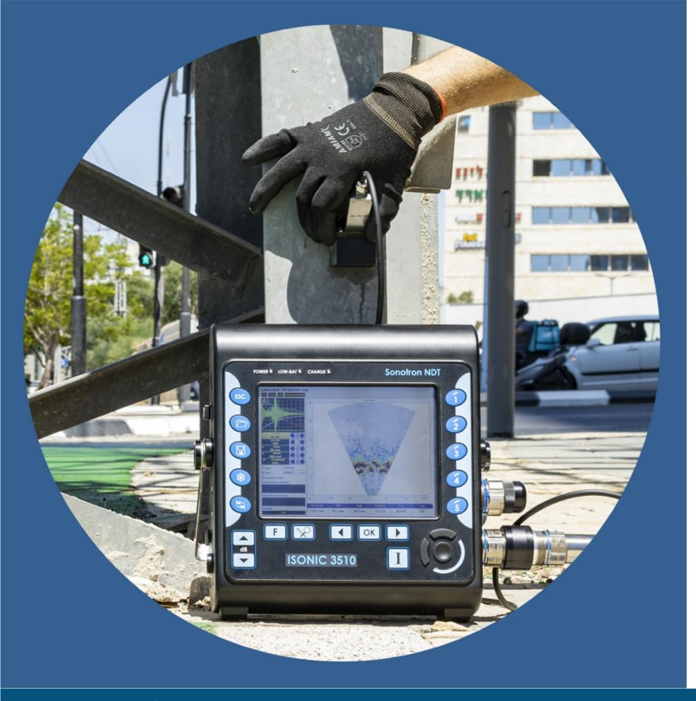
Short Range Guided Wave (SRUT GW) Inspection using Wedged Matrix Array Probes
